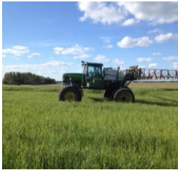
Figure 1. High clearance sprayer applying Headline EC Fungicide on perennial ryegrass near Churchbridge, SK in 2012. Source: Sorgard Seeds
